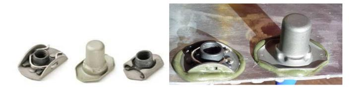
F: CN609 CN611 CN614 Nutplates Traditionally used in military or aerospace in place of a Nutsert where a floating nut is required to accept a screw or bolt. Common applications are electrical cabinets, sheet metal paneling. Sealed nutplates used in tanks as attachment points.
