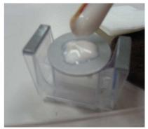
The fixture keeps the joint under constant pressure during the adhesive cure, and insures a consistent bond line.
