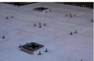
G: CB9522 Self fixturing stud, commonly know as the deckstud for its use on navy ships to attached ships deck boards, galley furniture and berths ECT. It has also been used to mount high stress applications due to its swivel base arrangement.
